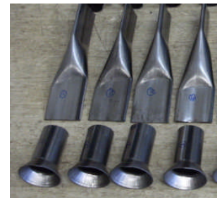
Weld Integrity Test Samples
